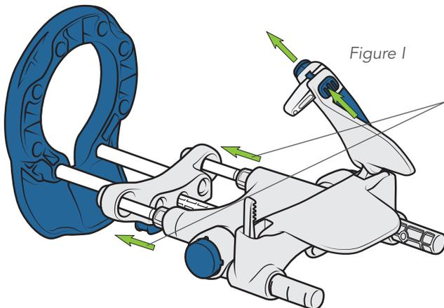
If it is difficult to release the clamp, push both rotation buttons simultaneously to return the RestoreX device to the straight position as depicted (*Figure I*) **or** move the main body along the tension rods toward the pelvic ring and lock into place. Now, open the clamp and remove the device.
